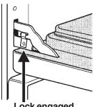
Lock engaged for door removal Figure 1
